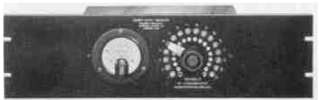
The TYPE 586 Power-Level Indicator program monitors the audio-frequency level fed to the transmitter
