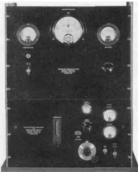
Visual indication of frequency deviation arrived in 1932 in the TYPE 581 Frequency-Deviation Meter
