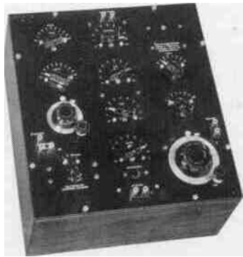
The latest development in measuring small inductances, the TYPE 667-A Inductance Bridge, June, 1935
