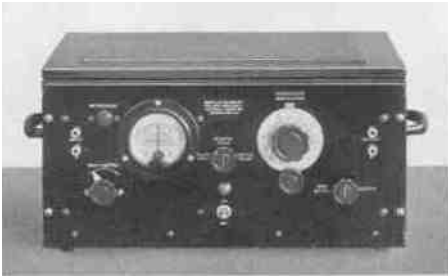
The Type 457 Modulation Meter gives laboratory measurement of percentage modulation on positive or negative peaks
