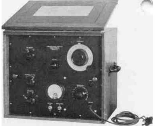
A simultaneous development for servicing and testing over a wide frequency range, the Type 601-A Standard-Signal Generator of July, 1931
