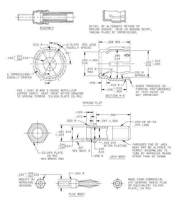
FIGURE C-2. Locking jack and plug for magnetron tubes.
