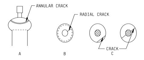
FIGURE D-2. Cracks.
