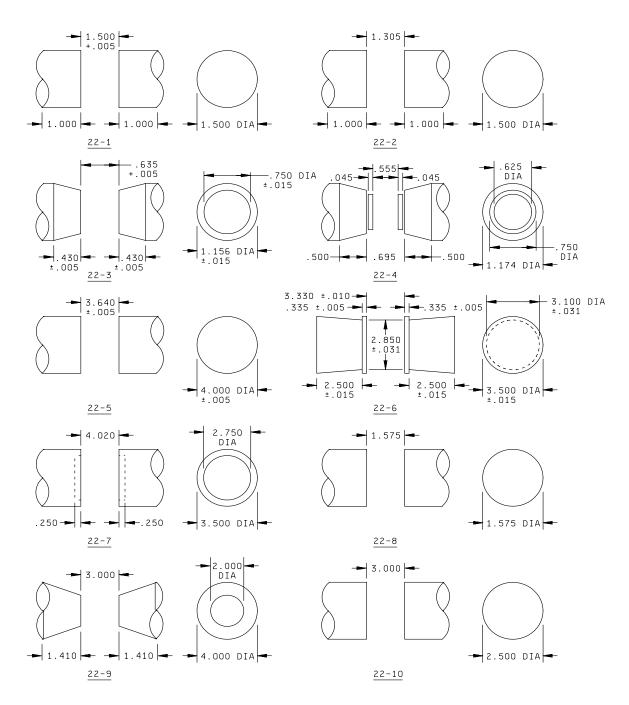
FIGURE C-1. Pole tips and gaps for magnetron tubes.
