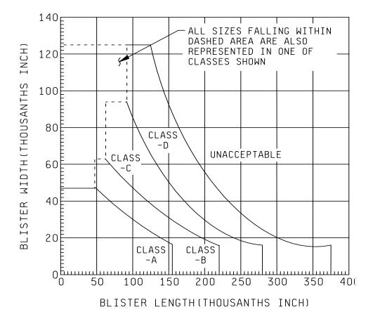
FIGURE D-1. Classification of soft glass unbroken blister sizes.
